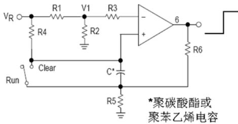
Time (t) =  $R4 C_n (V_R/V_R - V_i)$ ,  $R3 = R4$ ,  $R5 = 0.1 R6$
